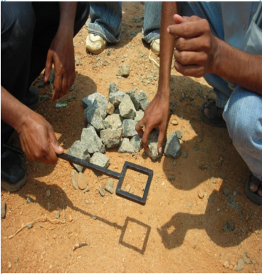
CMATs checking the size of the aggregates
